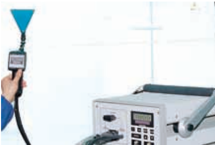
Integrity testing of HEPA filters
