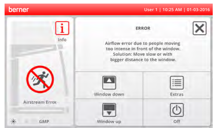
ALARM NOTICE IN DISPLAY Clear warning notice with red header and pictogram and proposed solution. "Info"-Icon for additional information on the situation.
